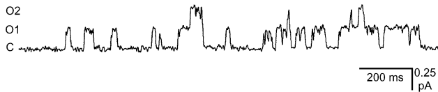
Fig. 1. Channel record from a typical patch clamp experiment in which two channels were active. The recording was made at +120 mV with 0.1 \mu M PF4 in the patch pipette. The signal was filtered at 1 kHz prior to digitisation, and at 100 Hz before analysis.
